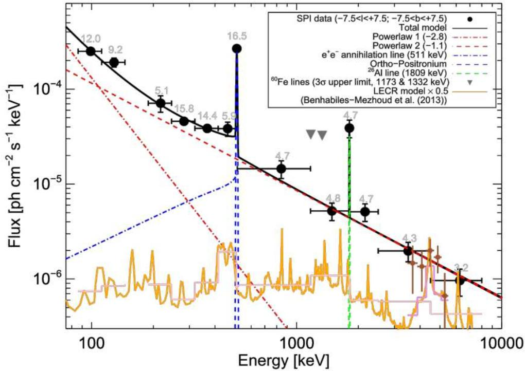
**Fig. 3.** SPI broadband spectrum of the inner Galaxy ( $|b| < 7.5^\circ, |l| < 7.5^\circ$ ). Shown is a **preliminary** analysis (black data points) from 14 years of SPI data, fitted by a phenomenological model (solid black line, individual components dashed coloured), and a prediction (orange, Benhabiles-Mezhoud et al. 2013) from CR excitation emission (Siebert et al. 2019, in prep.).
